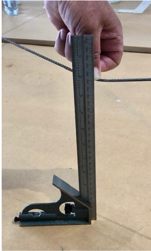
Photo 4. Measuring the sag of the wire rope. 250mm +/- 10mm.
