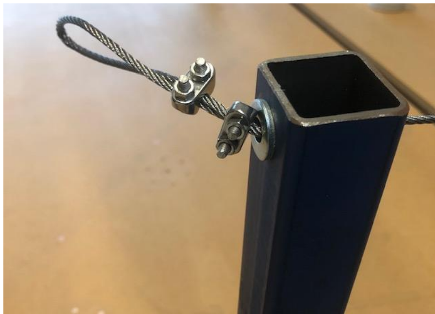
Photo 6. Wire rope/pylon/grips/washer assembly. Preferably, there is no gap between the two grips.
