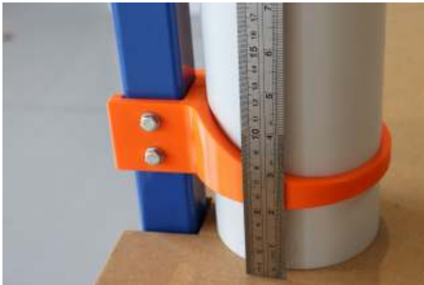
Photo 1. Lower silo bracket mounting location and orientation.
