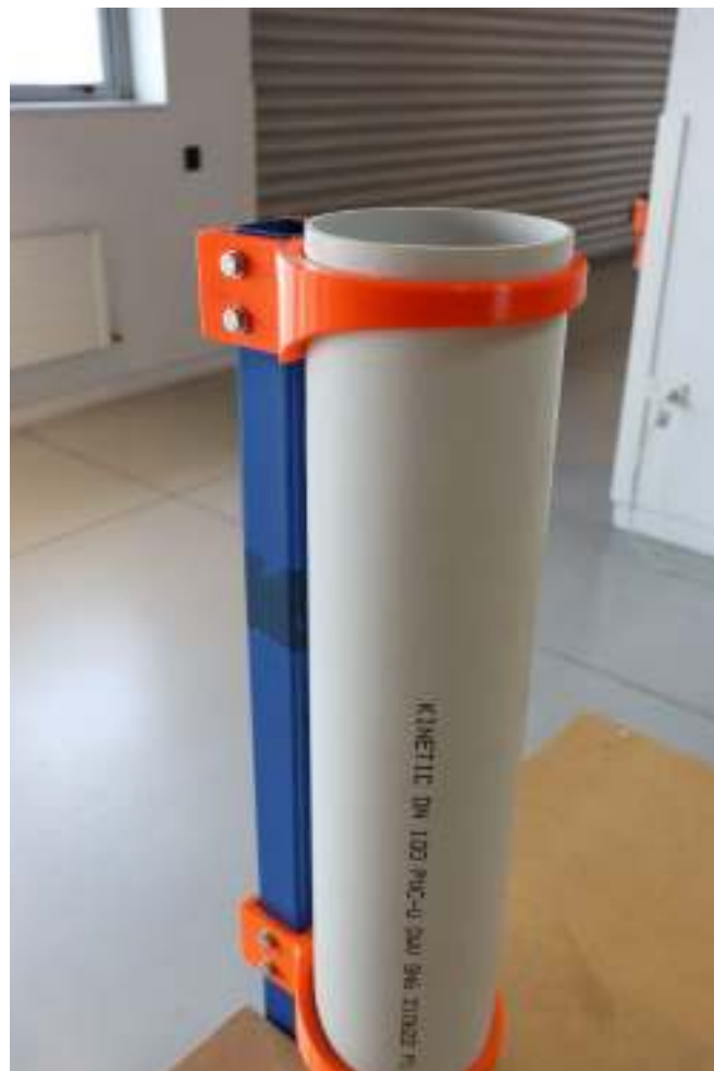
Photo 2. Pylon, bracket and silo assembly.
